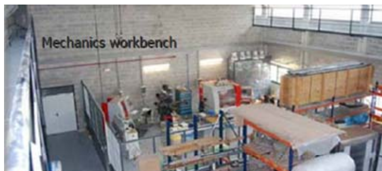
CNC lathers and grinders with ~5µm precision MIG and TIG soldering machines, 3D CAD design Visual and contact CMM with ~ 1µm prec.
